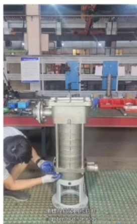
用螺栓拧紧四根拉杆 Tighten nut for rods.
