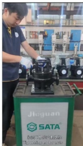
紧固电机座六颗螺栓 Tightening motor nuts.
