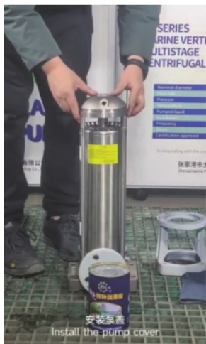
安装泵盖 Install the pump cover
