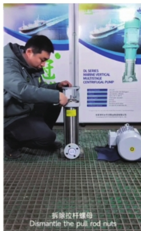
拆除拉杆螺母 Dismantle the pull rod nuts
