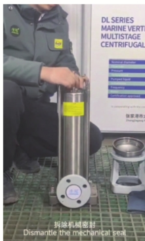
拆除机械密封 Dismantle the mechanical seal
