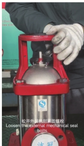
拆除旧机械密封，在原处上安装新机械密封 Dismantle old mechanical seal, then install new mechanical seal assembly on pump cover.
