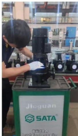
安装联轴器 Installation the coupling.
