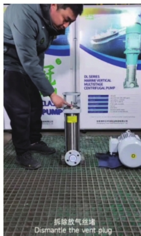
拆除放气丝堵 Dismantle the vent plug
