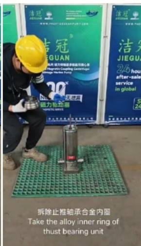
拆除止推轴承合金内圈 Take the alloy inner ring of thrust bearing unit
