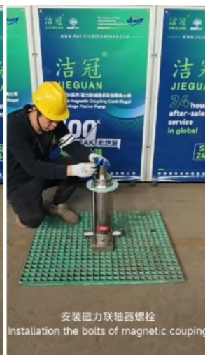
安装磁力联轴器螺栓 Installation the bolts of magnetic coupling
