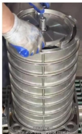
安装轴承导叶 Installation bearing guide impeller.
