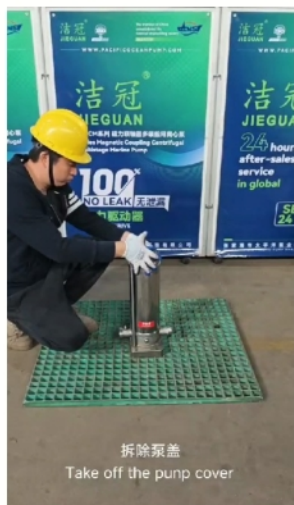
拆除泵盖 Take off the pump cover thrust bearing unit
