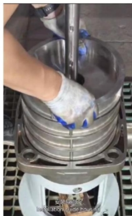
安装导流壳 Installation guide housing.
