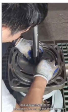
将平键安装到泵轴槽口处
