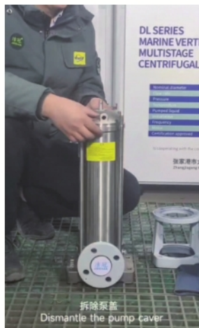
拆除泵盖 Dismantle the pump cover
