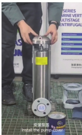
安装泵盖 Install the pump cover
