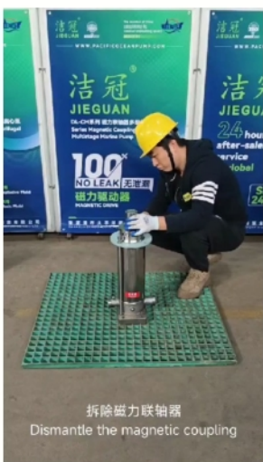
拆除磁力联轴器螺栓 Dismantle the magnetic coupling bolts
