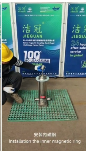
安装内磁钢 Installation the inner magnetic ring
