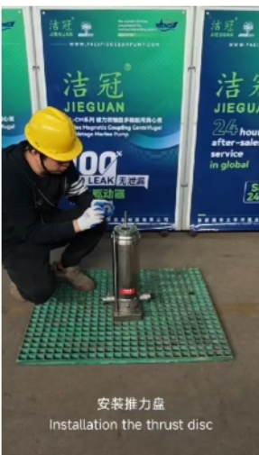
安装推力盘 Installation the thrust disc
