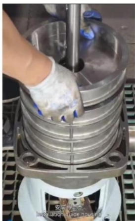
安装导流壳 Installation guide housing.
