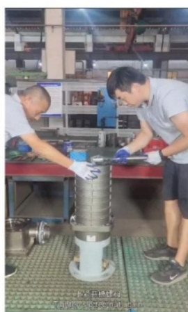
上紧开槽螺母 Tighten slotted nut again.
