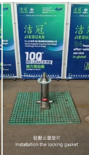
轻敲止退垫片 Installation the locking gasket
