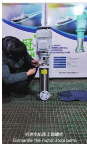
拆除电机座上端螺栓 Dismantle the motor stool bolts
