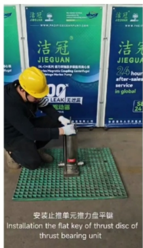
安装止推单元推力盘平键 Installation the flat key of thrust disc of thrust bearing unit
