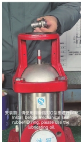
拆除旧机械密封，在原处上安装新机械密封 Dismantle old mechanical seal, then install new mechanical seal assembly on pump cover.
