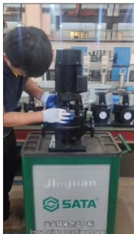
安装联轴器定位销 Installation coupling dowel.
