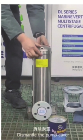
拆除泵盖 Dismantle the pump cover
