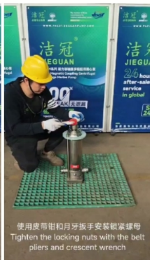
使用皮带钳和月牙扳手安装锁紧螺母 Tighten the locking nuts with the belt
