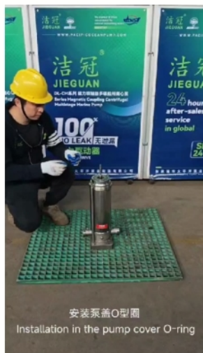
安装泵盖O型圈 Installation in the pump cover O-ring bearing unit
