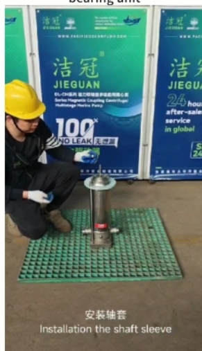
安装轴套 Installation the shaft sleeve magnetic ring
