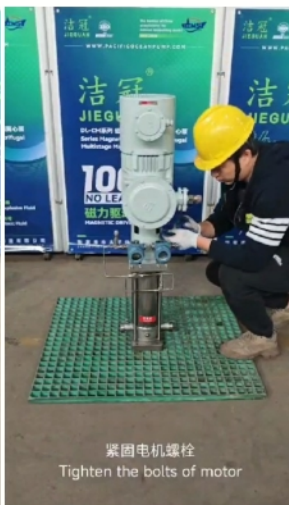
紧固电机螺栓 Tighten the bolts of motor
