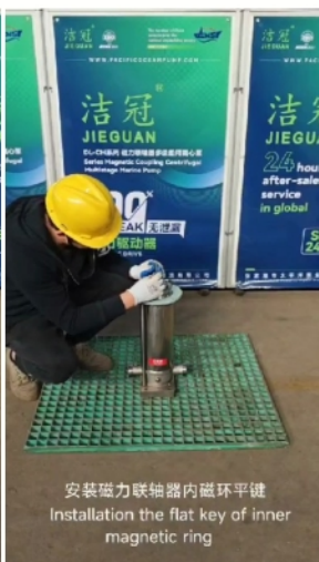
安装磁力联轴器内磁环平键 Installation the flat key of inner magnetic ring
