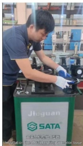
安装电机座处O型圈 Installation the O rubber ring at motor base.
