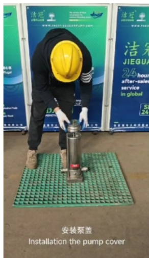
安装泵盖 Installation the pump cover magnetic ring
