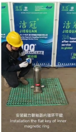
安装磁力联轴器内磁环平键 Installation the flat key of inner
