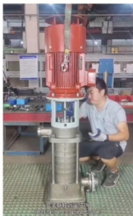
安装联轴器定位销 Installation coupling dowel.
