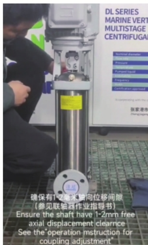
确保有1-2毫米轴向位移间隙 (参见联轴器作业指导书) Ensure the shaft have 1-2mm free axial displacement clearance See the "operation instruction for coupling adjustment"
