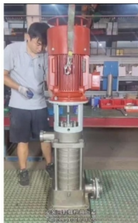
安装四颗螺栓并上紧 Tighten motor nuts.
