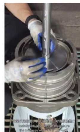
安装长级套， 长级套槽口对准泵轴槽口 Installation long sleeve make sure the key-way with shaft key-way.
