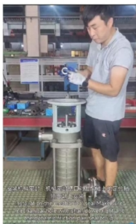
安装机械密封，机械密封槽口与轴上的定位销，镜面朝上安装。 Installation the mechanical seal, make sure mechanical hole with shaft dowel right and the dynamic friction pair seat to up.
