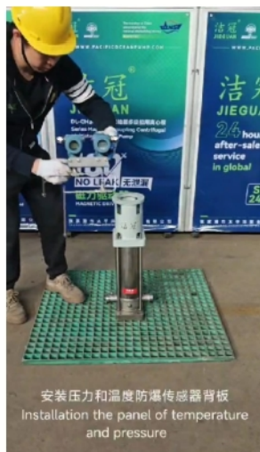
安装压力和温度防爆传感器背板 installation the panel of temperature and pressure
