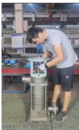
安装机械密封盖，并上紧螺栓。 Installation mechanical cover and Tighten nuts.
