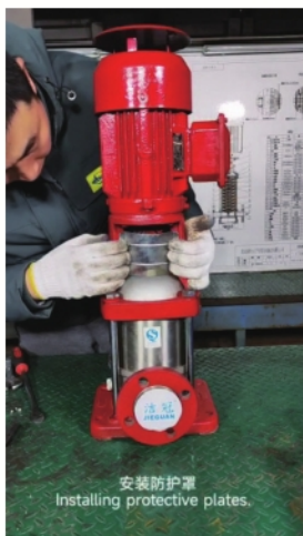
安装防护罩 Installing protective plates.
