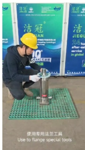
拆除磁力联轴器螺栓 Dismantle the magnetic coupling bolts
