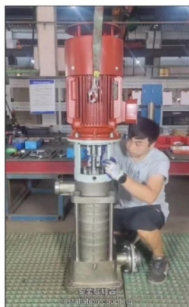
安装联轴器 Installation coupling.
