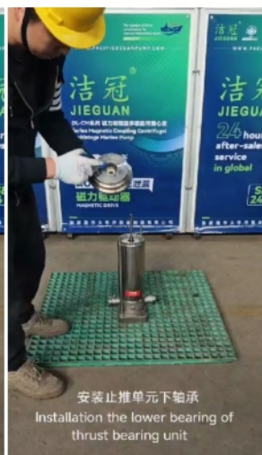
安装止推单元下轴承 installation the lower bearing of thrust bearing unit
