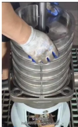
安装导流壳 Installation guide housing.
