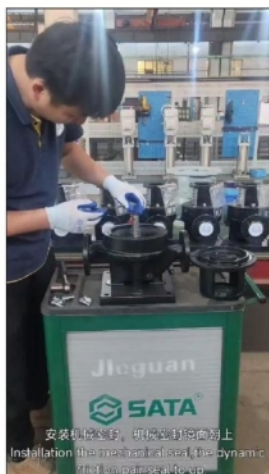
安装机械密封，机械密封镜面朝上 Installation the mechanical seal, the dynamic friction pair seal to up.
