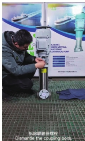
拆除联轴螺栓 Dismantle the coupling bolts
