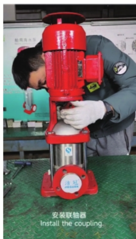
将电机重新装上，紧固螺栓 Installing the motor tighten the bolts.
