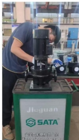
安装四颗螺栓并上紧 Installation motor nuts.
