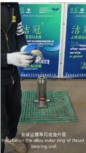
安装止推单元合金外圈 Installation the alloy outer ring of thrust bearing unit
