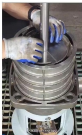
安装平键 Installation the key.
