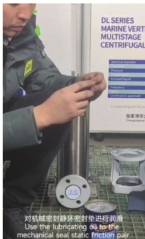
对机械密封静环密封垫进行润滑 Use the lubricating oil to the mechanical seal static friction pair
