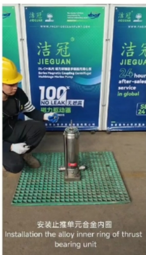
安装止推单元合金内圈 Installation the alloy inner ring of thrust bearing unit
