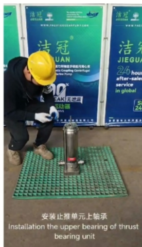
安装止推单元上轴承 Installation the upper bearing of Thrust bearing unit
