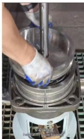
安装导流壳 Installation guide housing.
