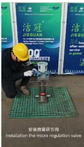
安装微量调节阀 Installation the micro regulation valve
