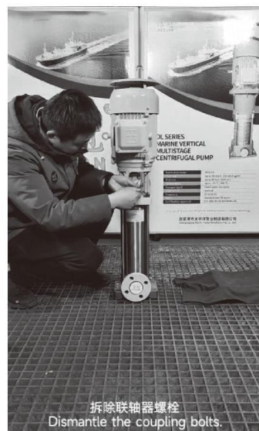
拆除联轴器螺栓 Dismantle the coupling bolts
