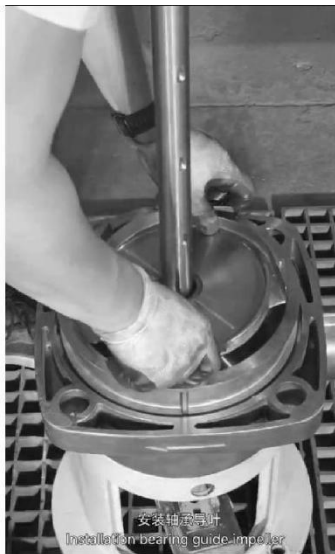
安装轴承导叶 Installation bearing guide impeller.
