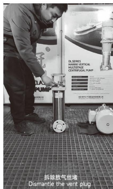
拆除放气丝堵 Dismantle the vent plug
