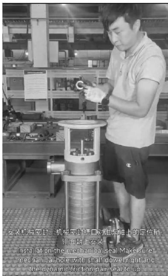
安装机械密封，机械密封槽口对准泵 轴上的定位销，镜面朝上安装。 Installation the mechanical seal, make sure mechanical hole with shaft dowel right and the dynamic friction pair seat to up.
