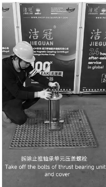
拆除止推轴承单元压盖螺栓 Take off the bolts of thrust bearing unit and cover
