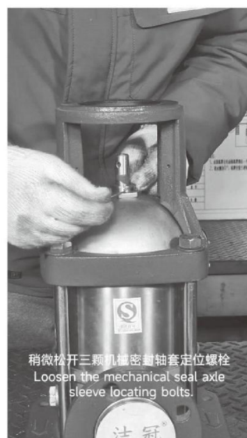
稍微松开三颗机械密封轴套定位螺栓 Loosen the mechanical seal axle sleeve locating bolts.
