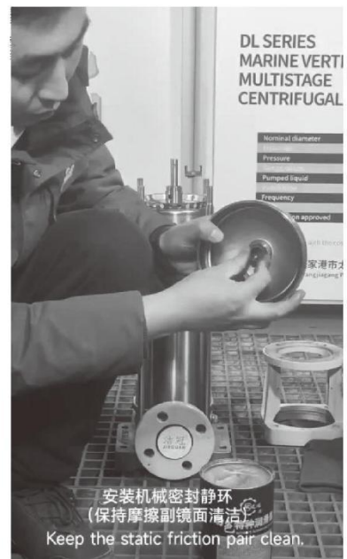
安装机械密封静环(保持摩擦副镜面清洁) Keep the static friction pair clean.
