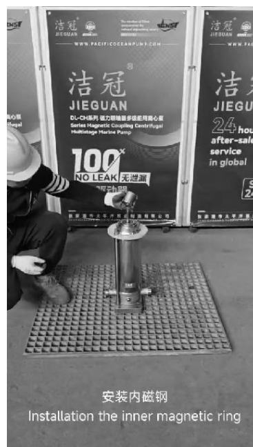
安装内磁钢 Installation the inner magnetic ring
