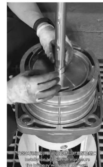
安装长间级套， 长间级套槽口对准泵轴槽口 Installation long stage sleeve make sure the key-way with shaft key-way.
