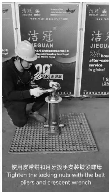
使用皮带钳和月牙扳手安装锁紧螺母 Tighten the locking nuts with the belt pliers and crescent wrench
