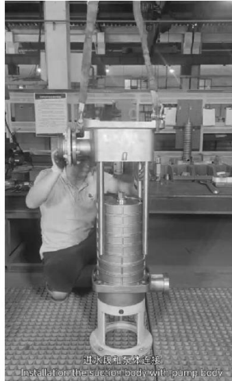
进水段和泵体连接 Installation the suction body with pump body.
