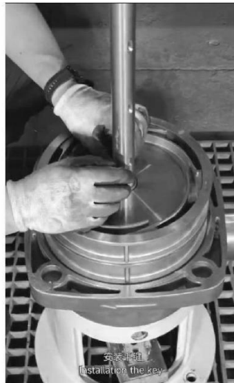
安装平键 Installation the key.
