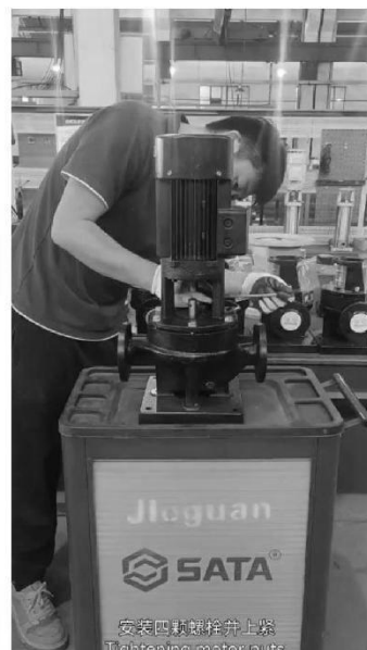
安装四颗螺栓并上紧 Installation motor nuts.
