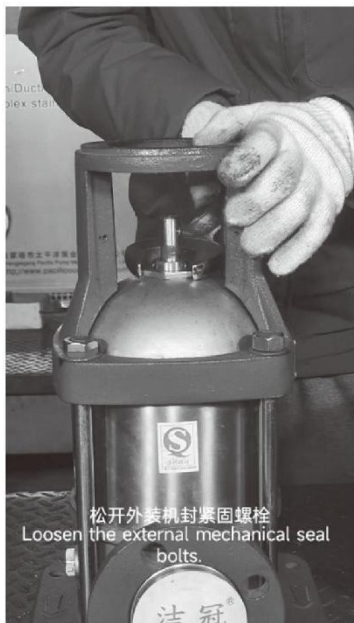
松开外装机封紧固螺栓 Loosen the external mechanical seal bolts.
