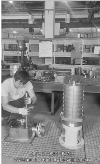
在进水段上安装四根拉杆 Installation four rods on the suction body.
