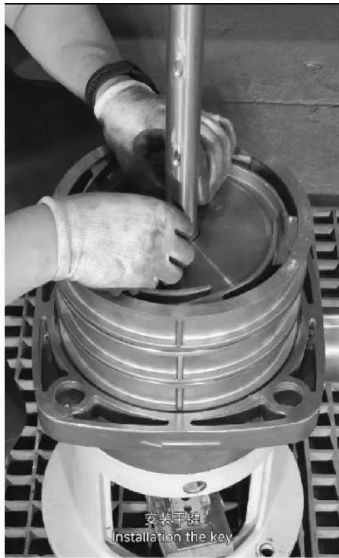
安装平键 Installation the key.
