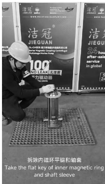
拆除内磁环平键和轴套 Take the flat key of inner magnetic Ring and shaft sleeve
