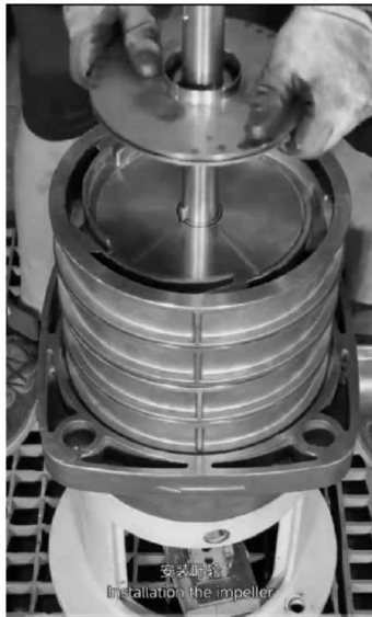
安装叶轮 Installation the impeller.
