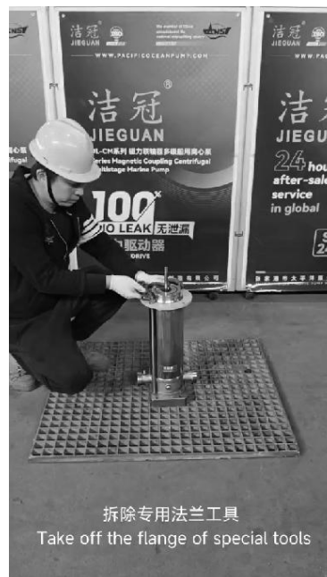
拆除专用法兰工具 Take off the flange of special tools
