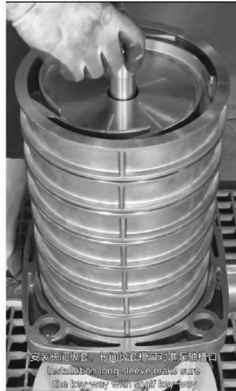
安装长间级套， 长间级套槽口对准泵轴槽口 Installation long sleeve make sure the key-way with shaft key-way.
