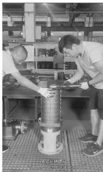
上紧开槽螺母 Tighten slotted nut again.
