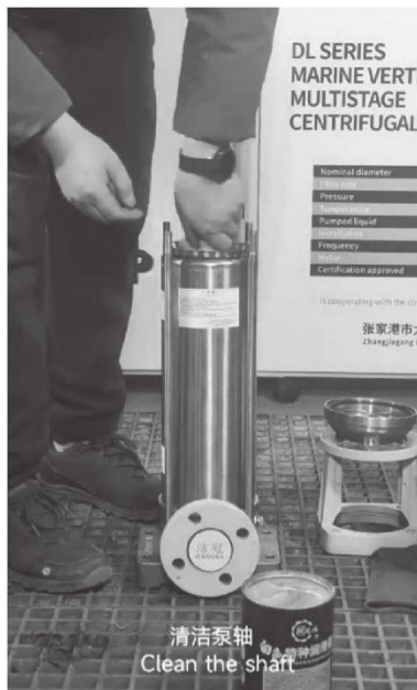
清洁泵轴 Clean the shaft
