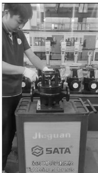
紧固电机座六颗螺栓 Tightening motor nuts.
