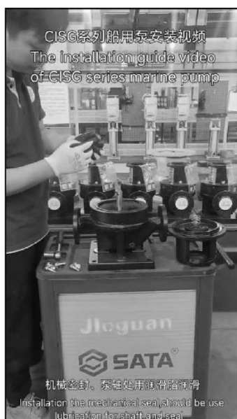
机械密封、泵轴处用润滑脂润滑 Installation the mechanical seal, should be use lubrication for shaft and seal.
