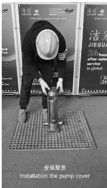
安装泵盖 Installation the pump cover
