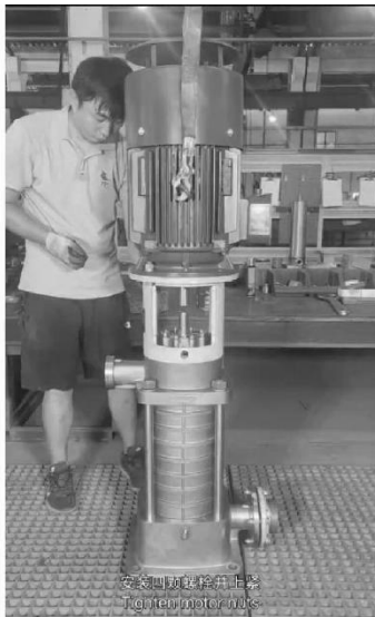
安装四颗螺栓并上紧 Tighten motor nuts.
