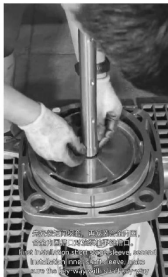
先安装短间级套，再安装合金内圈， 合金内圈槽口对准泵轴平键槽口。 First installation short stage sleeve, second installation inner shaft sleeve, make sure the key-way with shaft key-way.
