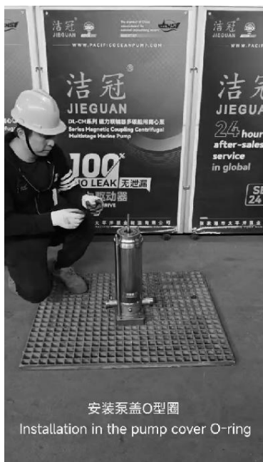
安装泵盖 O 型圈 Installation in the pump cover o-ring
