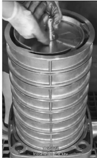
安装平键 Installation the key
