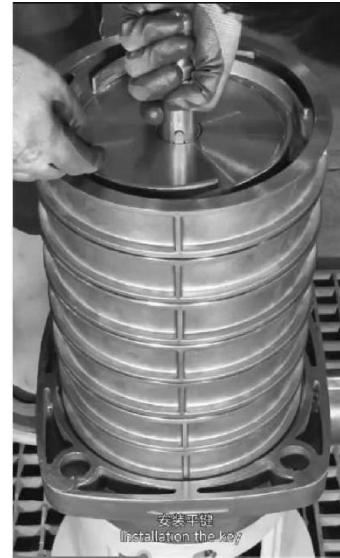
安装平键 Installation the key.
