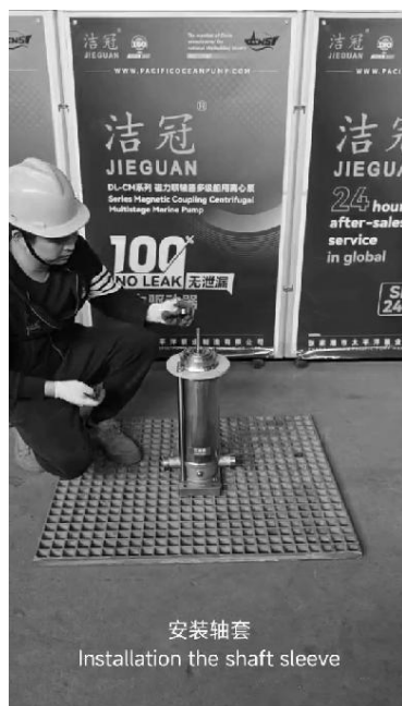
安装轴套 Installation the shaft sleeve
