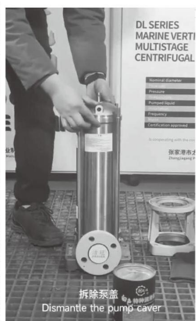
拆除泵盖 Dismantle the pump cover
