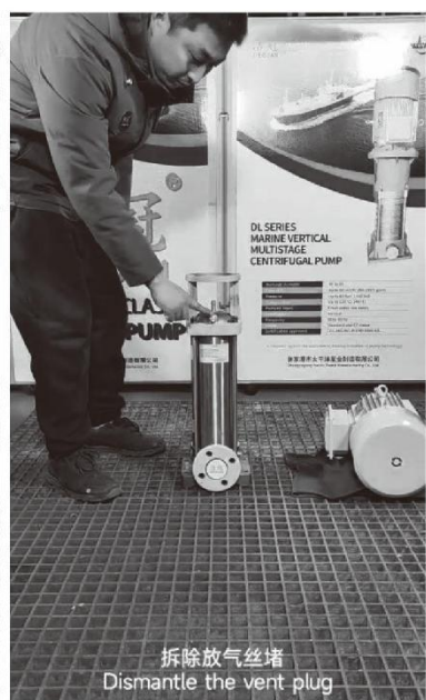
拆除放气丝堵 Dismantle the vent plug
