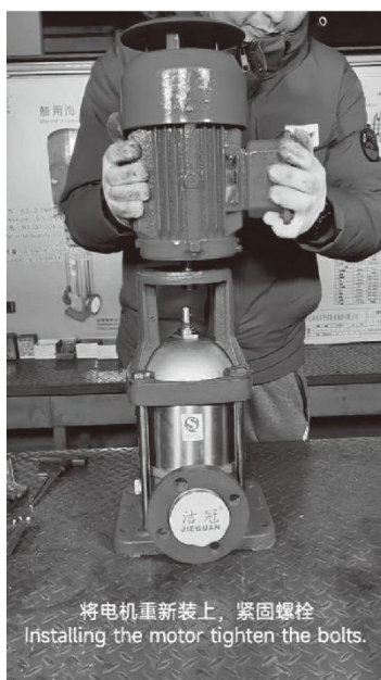
将电机重新装上，紧固螺栓 Installing the motor tighten the bolts.
