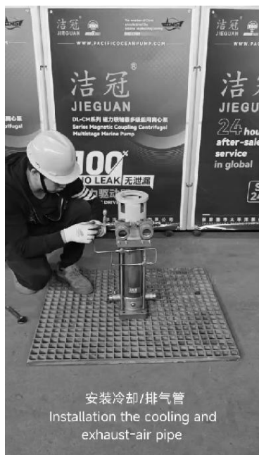
安装冷却/排气管 Installation the cooling and exhaust-air pipe
