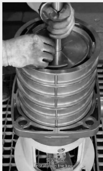
安装平键 Installation the key.
