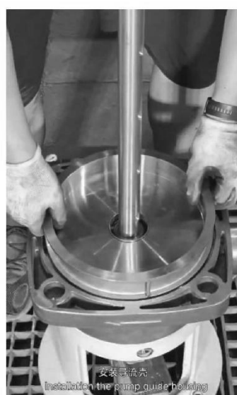
安装导流壳 Installation the pump guide housing.
