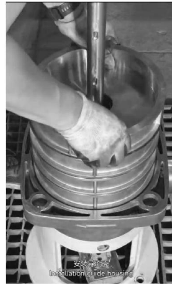
安装导流壳 Installation guide housing.
