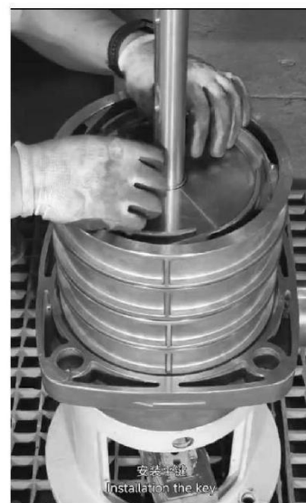
安装平键 Installation the key.
