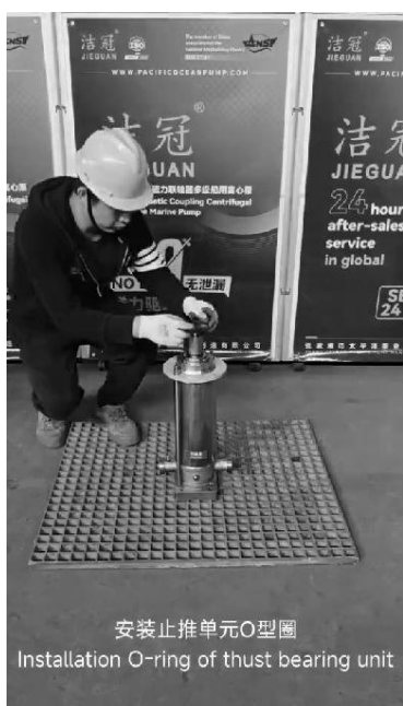
安装止推单元O型圈 Installation O-ring of thrust bearing unit
