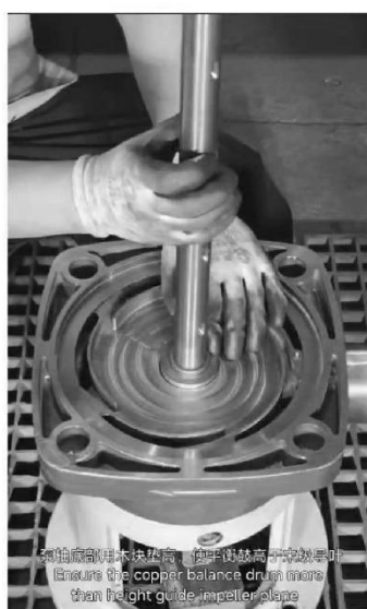
泵轴底部用木块垫高， 使平衡鼓高于末级导叶 Ensure the copper balance drum more than height guide impeller plane.
